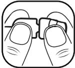
Squeeze the base of the tip while securing the speaker housing. Separate with a quick pull motion. Discard old earplug tip.
