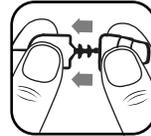
Holding the base of the new tip, press the speaker securely. Click into place.
